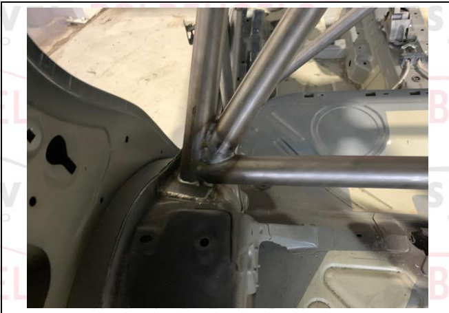
PHOTO 5 REAR BACKSTAY TO BODYSHELL ATTACHMENT
