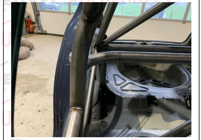
PHOTO 13 SHOULDER HARNESS ATTACHMENT - CO DRIVER
