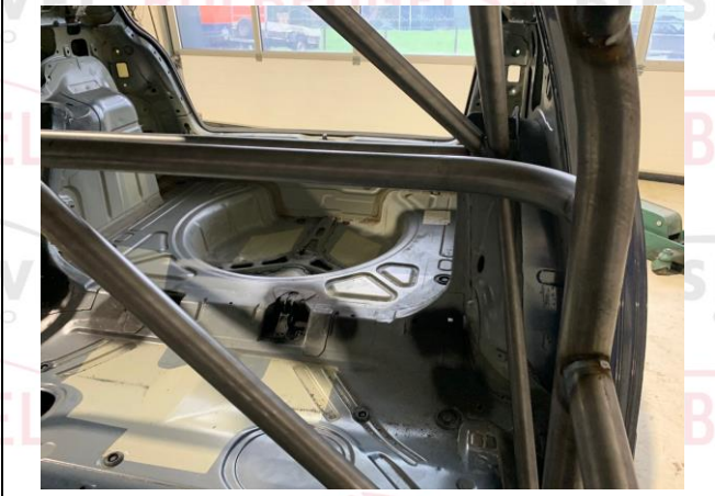
PHOTO 12 SHOULDER HARNESS ATTACHMENT - DRIVER
