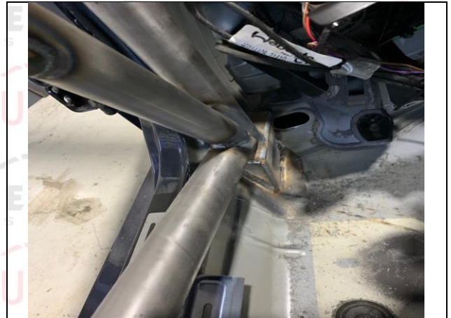
PHOTO 6 FRONT ROLLBAR TO FLOOR ATTACHMENT
